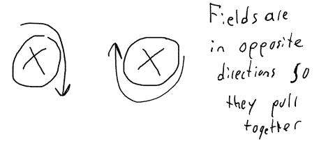
2. Two wires have current moving as shown, will the wires push each other apart or pull each other together?
