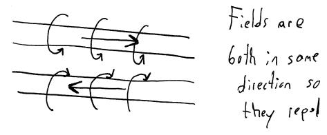
3. Two wires have current moving as shown, will the wires push each other apart or pull each other together?
