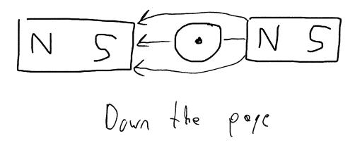
6. Determine the direction the wire shown will be pushed due to the magnetic field between the two permanent magnets shown.
