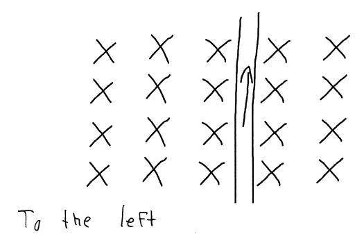
5. Which direction will the wire be pushed by the magnetic field created by the two permanent magnets shown.
